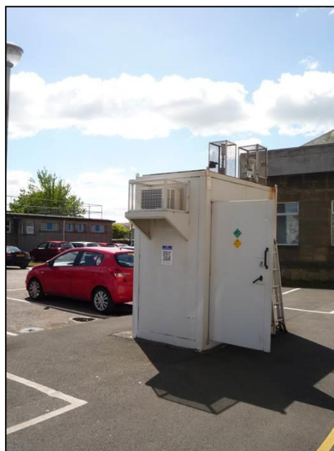
Figure 1. Example of an Automatic Urban and Rural Network station used to monitor Scotland's air quality. Thirty sampling sites were based around AURNs in Edinburgh.
